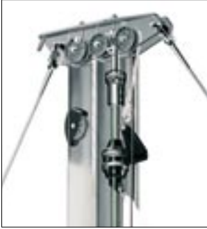
Seldén in-mast furling system: Geared line driver winch, tensioned luff extrusion, asymmetrical located sail slot and the patented load distributor of the halyard swivel. All to make furling an easy and fast operation.
